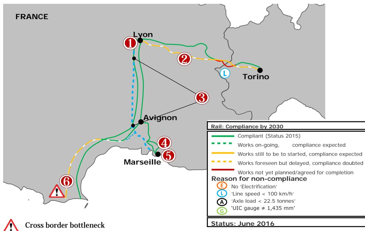
Figure 13 –French sections compliance by 2030 and main project impacting on KPI
